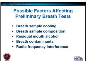
Radio frequency interference (RFI) can produce either high or low test results, or can prevent a breath test device from producing any result. Care should be exercised when utilizing a PBT around radio equipment.
